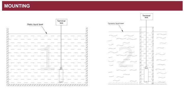
As shown in picture 1, when the sensor is installed in static water such as in poos, water towers, probe is immersed into the bottom and should be as far as possible away from the pump or valves. The terminal box should keep above water surface and prevent water penetrating into cables. Please make sure the airway not be blocked.
