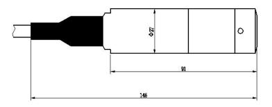
The default diameter is 27 mm. 19 mm or 13 mm external diameter is customizable.
